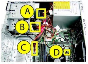
8. Disconnect the power cable from the optical disc and hard disk drives by squeezing the latch (1) on the connectors and pulling to remove.
